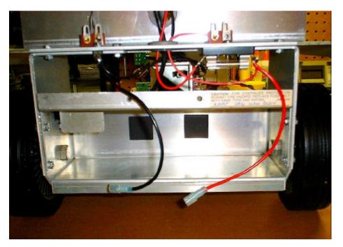
*NOTE:* You will notice two aluminum tabs that hang down into the battery compartment to keep the original batteries centered. In order to allow the new battery to be installed the one tab on the right (as viewed from the front) needs to be bent up out of the way. This can often be done by hand.
